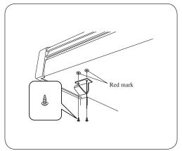
6. Turn the Adjuster (installed on the bottom of C) until it touches the floor to support the pedal board.
